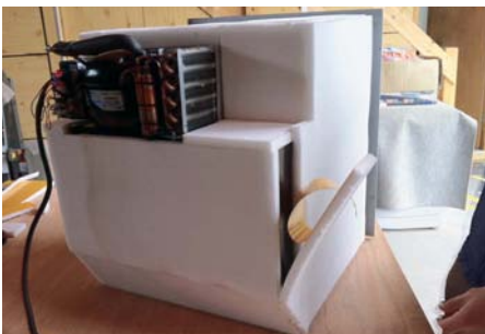
Motorhome fridges are a compromise between insulation levels and interior space
