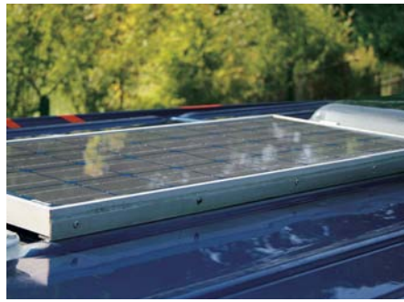
The solar panel was fitted between two roof vents
